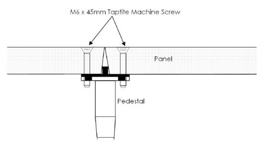
The Taptite TRILOB machine screw has a triangulated and tapered end on the screw thread so when screwed into the hole will self tap its own thread through the hole predrilled in the pedestal head.
